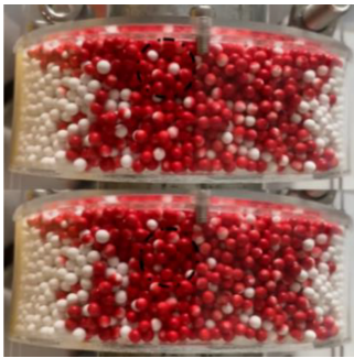
(b) “类液体”颗粒状态 (b) Liquid-like particle state
