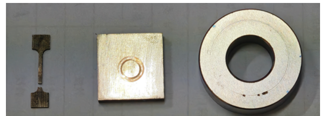
(a) 拉伸 (b) 摩擦磨损 (c) 滚动接触疲劳 (a) Tensile (b) Friction and wear (c) Rolling contact fatigue
