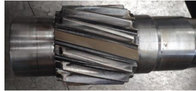
(c) 断齿故障小齿轮
