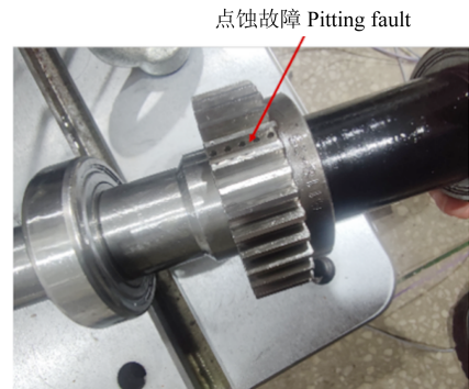
图9 点蚀故障齿轮
