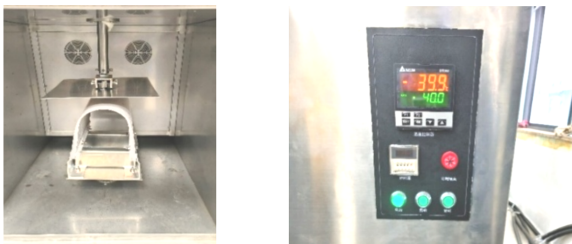
(a) 外风挡安装图 (a) Installation drawing of the outer windshield (b) 试验箱温度设置图 (b) Temperature setting diagram of test chambers
