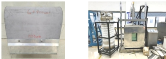
(a) U型橡胶外风挡样件 (a) U-shaped rubber outer windshield sample (b) 高低温试验箱 (b) High and low temperature test chambers
