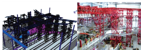
(a) 虚拟加载场景 (b) 试验现场照升 图 5 庞巴迪 Global7500 全机耐久性\损伤容限试验 [87] Fig. 5 Durability/Damage tolerance test [87] of Bombardier Global7500
