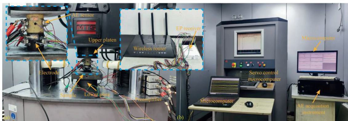
Fig. 1. Experimental test system for uniaxial compression test: (a) Uniaxial loading system, and (b) EP and AE recording systems.
