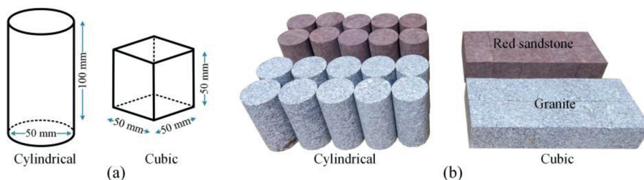
Fig. 2. Rock specimen. (a) Schematic diagram of basic dimensions, and (b) Photograph of specimen.
