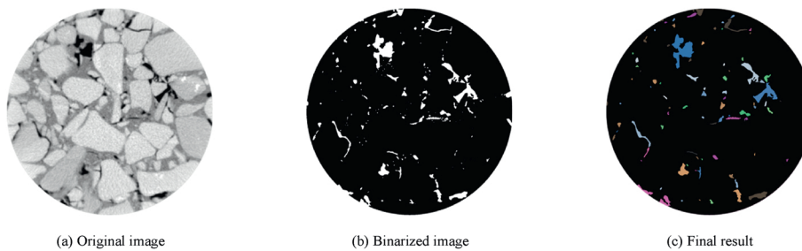
Fig. 5. Pore analysis images based on PCAS.
