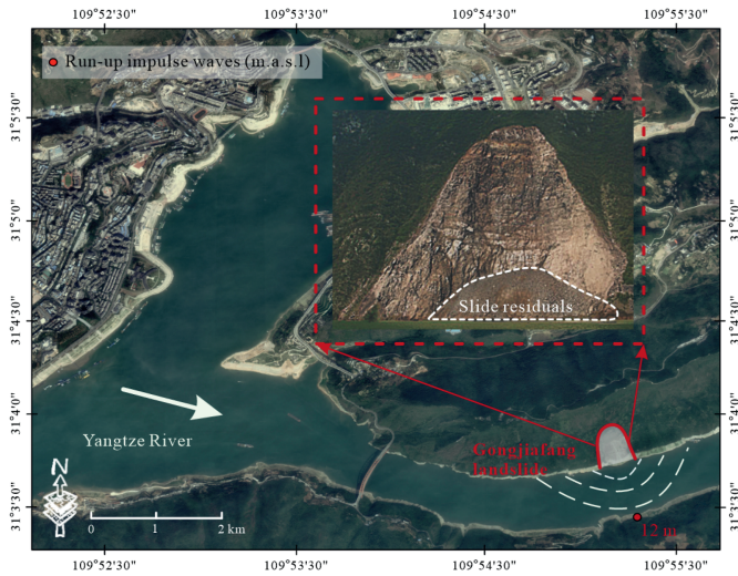
Fig. 9. The aerial photomosaic of Gongjiafang landslide occurring on November 23, 2008. The red dot is the recorded run-up height.
