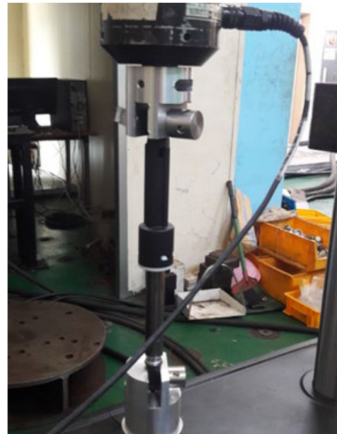
FIGURE 4 | The free-stroke damper test using a uniaxial test system.
