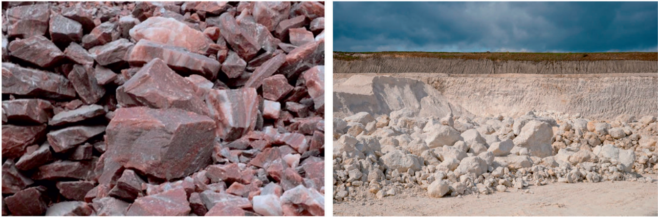
Fig. 1. Sample rockpiles with different shapes, left: more angular particles, right: more rounded particles.
