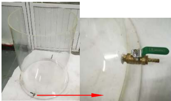
图3 试验所用模型箱及底部进水排水孔 Fig. 3 Model box and water inlet draining valve at bottom
