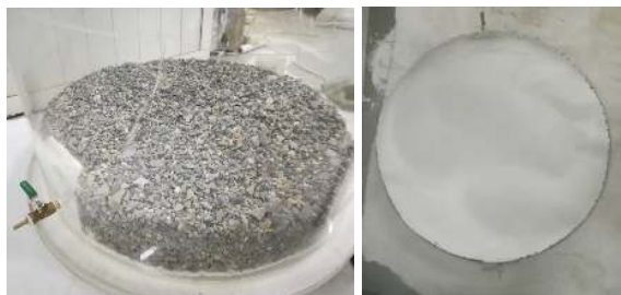
图4 铺设排水层、土工布和滤纸示意图 Fig. 4 Schematic diagram of laying the draining layer, geotextile and filter paper
