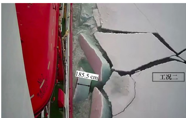
图 1 “雪龙”号科考船北极航行中的冰厚测量示例 [29] Fig. 1 Example of ice thickness measurement during the Arctic voyage of Xuelong scientific research ship [29]
