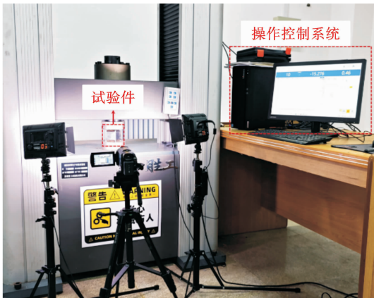
图 3 复合管件准静态轴压试验现场布置
