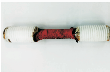
(a) 腐蚀60天锈蚀产物 (a) Corrosion products for 60 days
