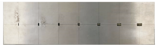
(b) 试件 2: 底部减薄缺陷 (b) Specimen 2: bottom thinning defects
