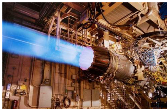
(b) Assessment of ceramic matrix composite nozzle in F135 engine
