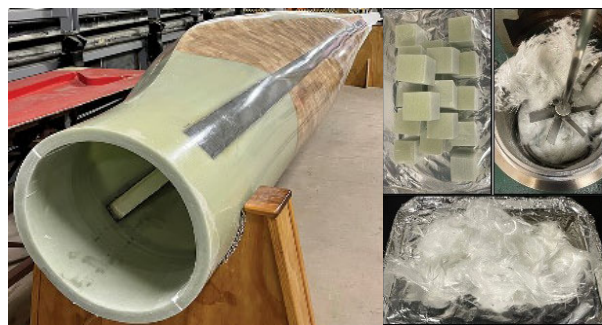
图 6 基于化学回收技术实现退役叶片材料中纤维的回收 [22] Fig. 6 Fiber recovery from decommissioned blade based on chemical recovery technology [22]
