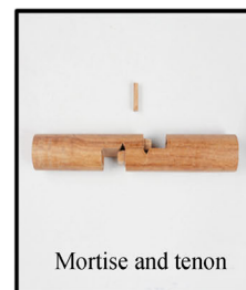
(b) Visual of the mechanical interlocking effect
