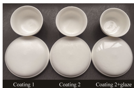
(c) Prestressed ceramic samples
