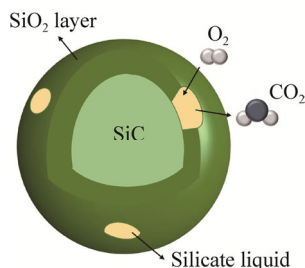
(c) Schematic diagram of SiC foaming reaction process at high temperature
