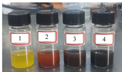
(a) Sealed Li_2S_6 /DME solution (1), after contact with Fe_2O_3 (2), Fe_2O_3@PPy-1 (3) and Fe_2O_3@PPy-3 (4)
