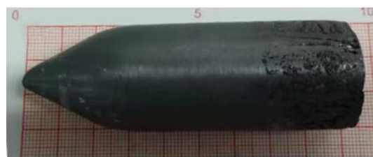
(a) Diagram of growing \text{Cd}_{0.9}\text{Mn}_{0.1}\text{Te:In/V} ingots ( \phi 30 \text{ mm} \times 95 \text{ mm} )
