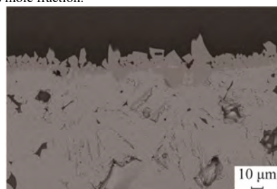
(a) (5\text{RE}_{0.2})\text{TaO}_4 after CMAS corrosion for 6 h
