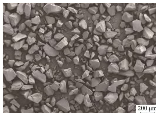
(c) Broken ceramic powder (50×)
