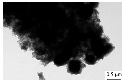
(c) TEM image of recycled \text{FeMnO}@C
