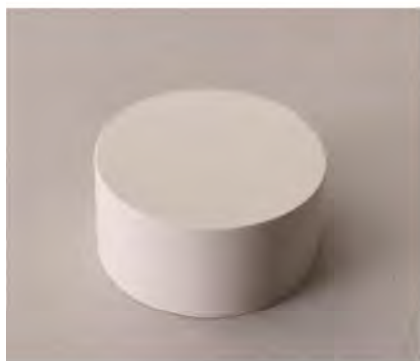
(a) Photograph of \text{TiO}_2 /PTFE composite
