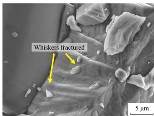
(a) Whiskers fractured
