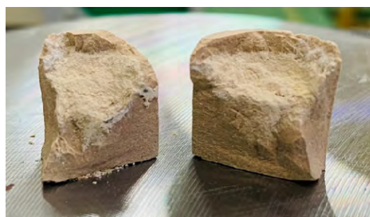
(b) Fracture of the carbonated Fe - \gamma - C_2S compacts with chitosan
