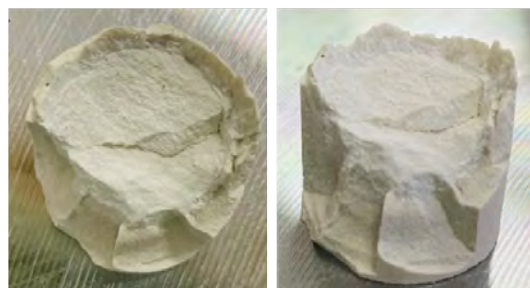
(a) Fracture of the carbonated \gamma - C_2S compacts with chitosan
