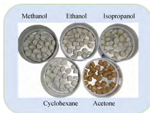
图 2 溶剂交换 7 d 后样品的外观特征 Fig. 2 Appearance characteristics of samples after solvent exchange for 7 d
