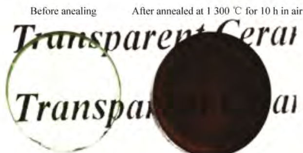
(b) Appearance of 0.3% Cr:YAG transparent ceramic before and after annealing
