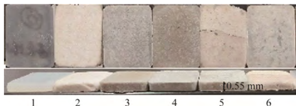
图 2 珍珠岩和气相 SiO 2 填充硅橡胶保温材料的照片 Fig. 2 Photographs of the perlite and fumed SiO 2 filled silicone rubber thermal insulating materials
