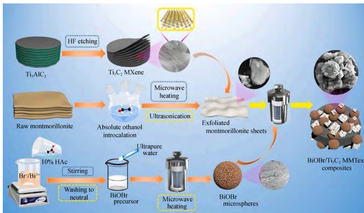
(a) Schematic representation for the preparation of BiOBr/Ti 3 C 2 /MMTex composite
