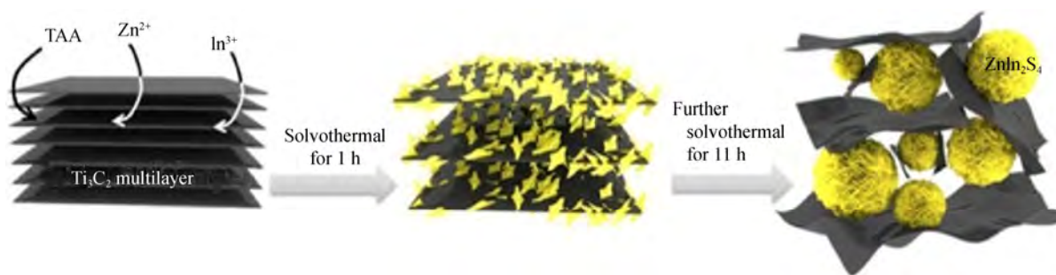
(b) Schematic representation for the preparation of ZnIn 2 S 4 /Ti 3 C 2 composite
