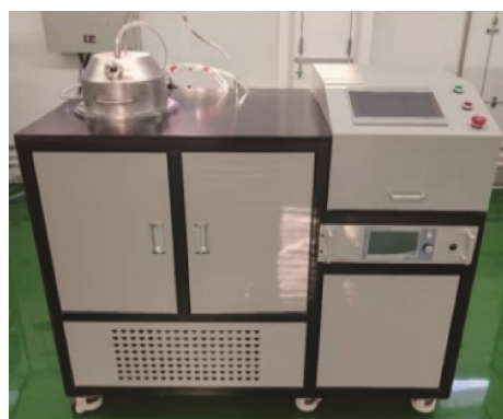
(a) Cap-shaped cavity type reactor, Harbin Institute of Technology(HIT)
