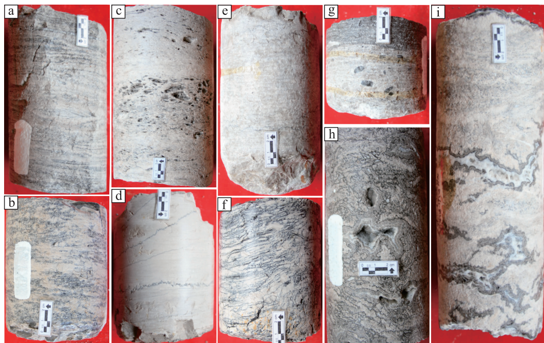
a—藻叠层白云岩，862.96~863.14 m；b—藻凝块白云岩，421.80~421.92 m；c—藻凝块白云岩，发育溶蚀孔洞，826.48~826.75 m；d—泥晶白云岩，可见缝合线，501.67~501.82 m；e—粉晶白云岩，524.61~524.80 m；f—含藻纹层泥晶白云岩，发育裂缝，沥青充填，518.13~518.25 m；g—砾屑白云岩，452.45~452.53 m；h—葡萄花边白云岩，发育溶洞，805~805.23 m；i—葡萄花边白云岩，胶结作用强烈，见晶间残余孔洞，853.62~853.92 m
