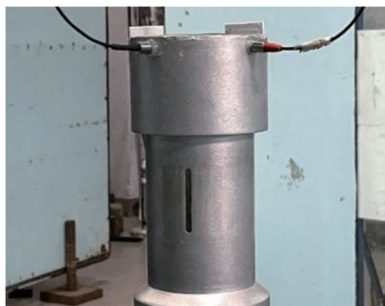
图 12 模型顶部加速度传感器布置 Fig. 12 Acceleration sensor layout at the top of the model
