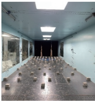
图 10 吸热塔模型风场布置照片 Fig. 10 Photos of wind field layout of solar tower model
