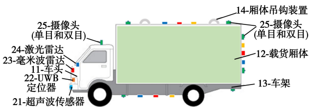
图 4 载货车辆结构布局和车载智能传感器布局设计 [20] Fig. 4 Structure layout of cargo vehicles and layout design of vehicle intelligent sensing sensors [20]
