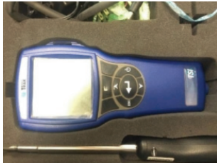
图 4 TSI 热线风速仪 Figure 4 TSL hot-wire anemometer
