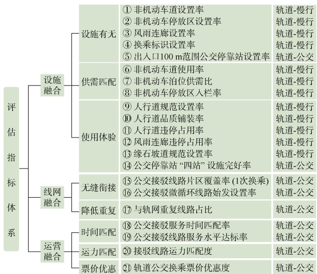
图 1 “轨道-公交-慢行”接驳评估指标体系 Figure 1 “Rail-bus-slow travel” connection evaluation index system
