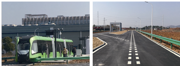
图 10 电子导向胶轮系统列车及其“虚拟轨道” Figure 10 Train of electronic guidance rubber-tired system and its “virtual track”
