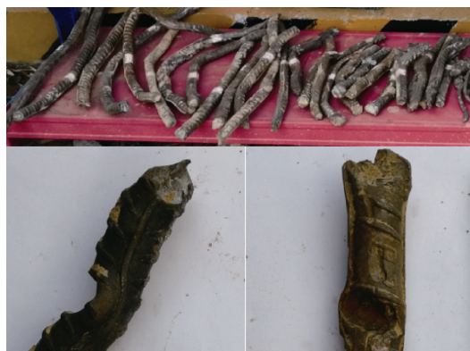
图 14 钢筋切口 Figure 14 Cutting of steel bars
