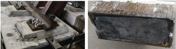
图 7 疲劳试验后轨道结构和灌注材料状态 Figure 7 Track structure and the grouting material status after the fatigue test
