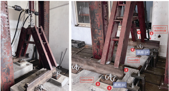
图 6 改造后轨道疲劳测试现场及测试点示意 Figure 6 Schematic diagram of the post-retrofitting track fatigue test site and test points
