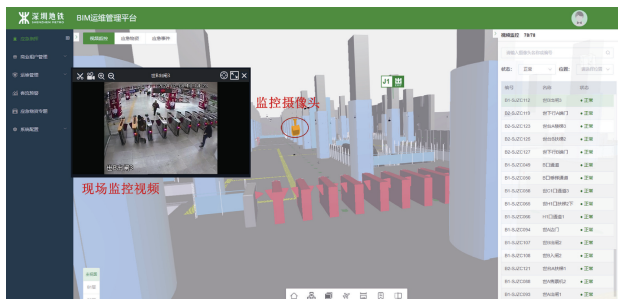
图 4 既有轨道交通项目 BIM 构件与现场匹配关系 Figure 4 Correlation between BIM components and site conditions in existing rail transit projects
