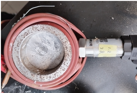
图 7 缸筒加热带及温度传感器 Figure 7 Cylinder heating band and temperature sensor
