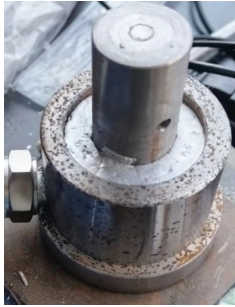
图 6 T70、T92 低熔点合金升降温受力性能试验加载缸筒 Figure 6 Loading cylinder for heating and cooling stress performance tests on T70 and T92 using low-melting-point alloys
