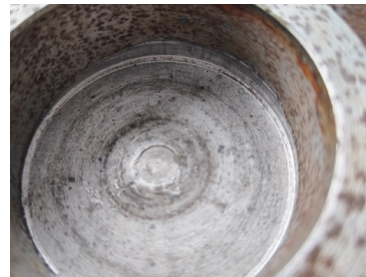
图 10 合金挤出痕迹 Figure 10 Extrusion trace of alloy
