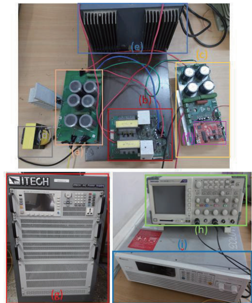
Fig. 15. Experimental setup with (a) PV-boost converter circuitry, (b) PSFB converter circuitry, (c) Totem-pole PFC converter circuitry, (d) L Filter (e) load, (f) Microcontroller- TMS320F28027F, (g) AC power supply, (h) DSO, (i) PV Simulator.
