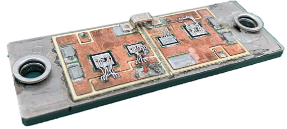
Fig. 2. Open-shelled IGBT module of Infineon FF50R12RT4.
