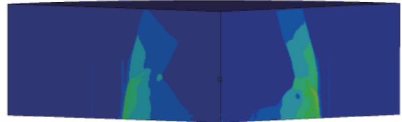
图8 椭圆-3药柱爆炸波阵面传播情况 Fig.8 Propagation of the explosion wavefront for elliptical-3 charge
