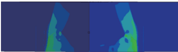
图6 椭圆-2药柱爆炸波阵面传播情况 Fig.6 Propagation of the explosion wavefront for elliptical-2 charge
