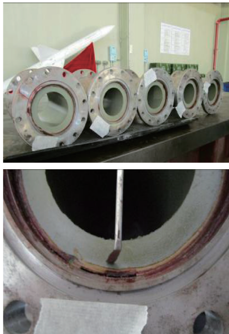
图8 预置缺陷标准试验发动机 Fig.8 Precast defects of standard testing motor
