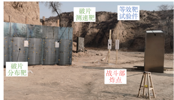
图10 等效靶毁伤试验现场布置
